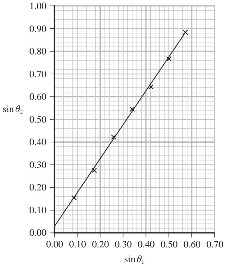
(i) Explain why the gradient of this graph can be used to determine the refractive index of the transparent material.
